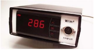
A continuous display of the solar irradiance directly in watts per square meter can be achieved by using the SolData type 104DM display module shown above.
